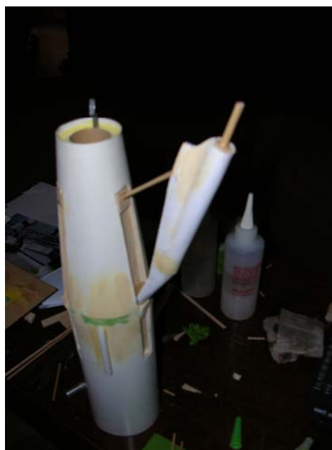
An almost completed landing gear. Typing paper wrapped around a dowel did the trick!
